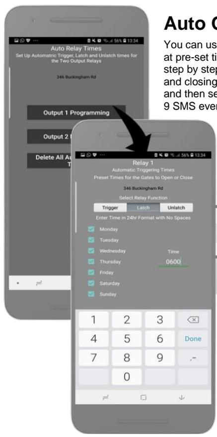
Toggle between trigger, latch and unlatch
