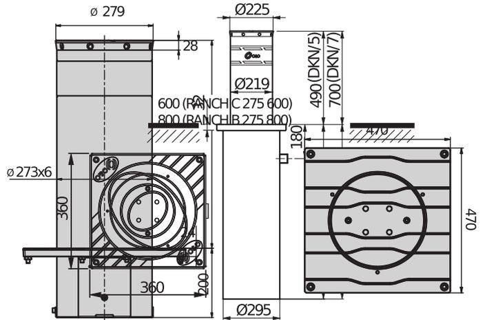
Fixed bollards used for preventing access for long periods. Bolted to the ground, their purpose is to block an access point or a road. They can integrate the use of automatic or semi-automatic bollards.
