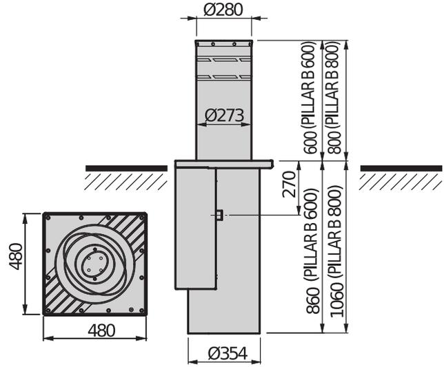
Anti-terrorist hydraulic bollard with incorporated hydraulic control unit. Suitable for protecting sensitive sites, thanks to the special "SD" version, which keeps the shaft raised in case of a power failure and with public installations where, in the standard version, the shaft lowers automatically with no power.
