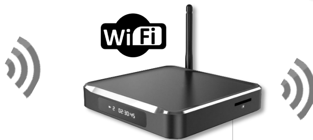
Long Range Antenna (2.4GHz) (up to 65 yards working range depending on router type and location)
