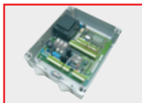
KD113693 00001 RIGEL 5 NO CAPACITORS Rigel 5 115 vac with built in 433 receiver
