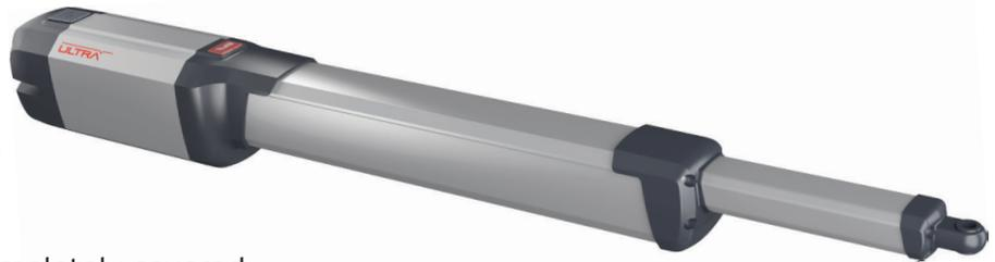
The advantage of the system is the completely covered screw drive with magnetic stops in the same enclosed housing. This ensures maximum protection against external agents (water, dust, dirt, etc.) as well as a total protection for people, preventing any type of access to the moving parts.
