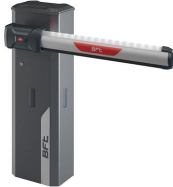
24V traffic barrier with a sturdy gearbox (all metal components) for clear passages up to 20'/6m. The U-Link control board with an LCD display allows a complete management of all the features and settings and it allows a simple integration of the traffic barrier with Parking or Building Management systems.
