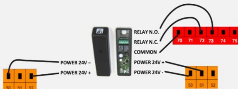
EXAMPLE 2: UL 325-2016 SAFETY PHOTO BEAM SENSOR WIRING
