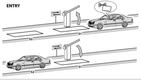
The recognition system enables barrier opening. If the coil **S1** is not occupied within the
