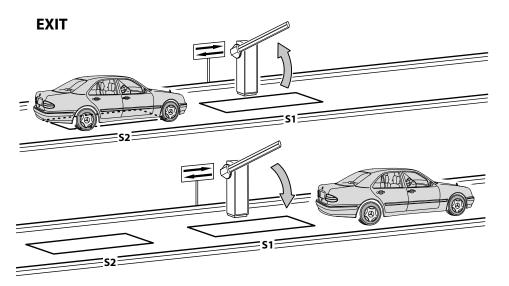
The vehicle approaches the reserved area. When the coil **S2** is occupied, barrier opening is enabled. If the coil **S1** is not occupied within the pause time, the barrier closes again.
