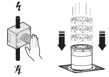
The deterrent bollard lowers spontaneously when you disconnect the power supply.
