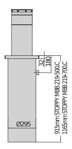
Complete range of automatic electromechanical retractable bollards for the protection and safety of all areas that require controlled access. Rod height 500 and 700mm. Ideal for contexts of particular architectural interest, guaranteeing maximum reliability over time and requiring minimal maintenance.
